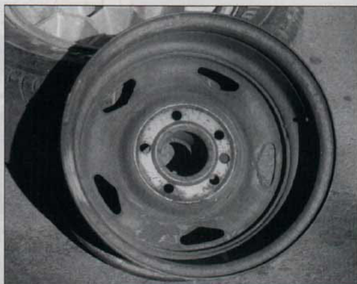
Note the unique steel wheel to which the polycast fascia was affixed. The 14-inch and 15-inch wheel look much the same, save diameter.
