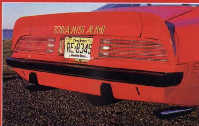
At the rear, the correct twin exhaust tips emit the raucous tones of the torque monster SD-455 with the sound tuned by a Flowmaster muffler.
